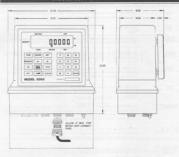
ACCURACY: ±1% of applied loads or one weight increment, whichever is greater.
